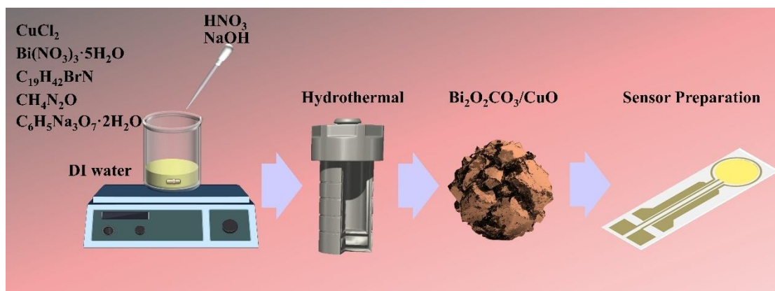
Figure 6-1 Schematic illustrations of the fabrication process of C_{ux} -BC microstructure.
